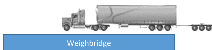
Figure 11: Semitrailer and dolly weighed with dolly off the weighbridge
